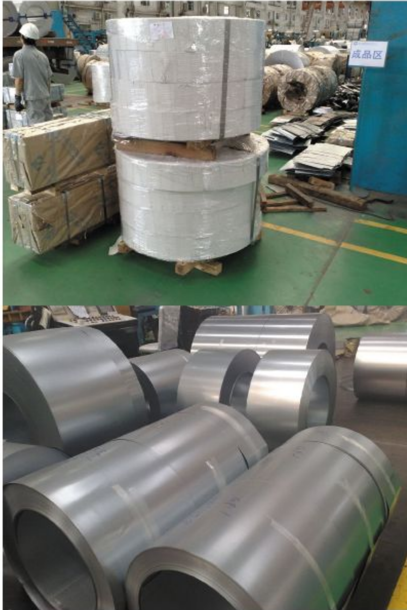
Steel sheets after slitting and shearing
