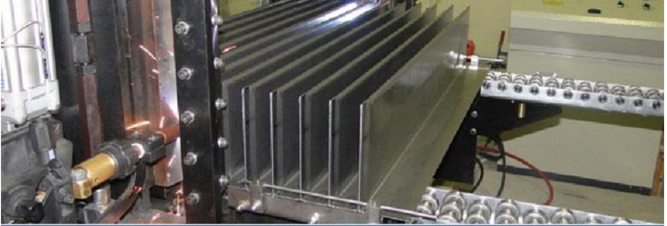
WELDING PROCESS OF CORRUGATED WALLS
